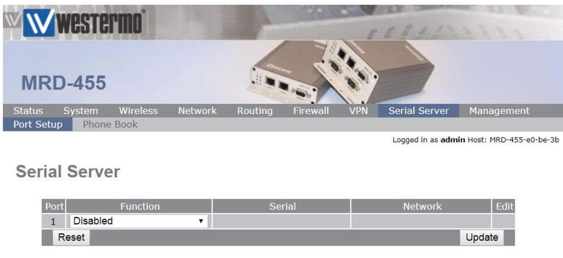
The screenshot shows the MRD-455 web interface. The navigation menu includes Status, System, Wireless, Network, Routing, Firewall, VPN, Serial Server, and Management. The 'Serial Server' section is active, and the 'Port Setup' sub-tab is selected. The main content area shows a table for configuring serial ports:
